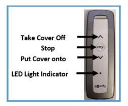
Note: User will identify on site that up and down arrows will change depending on orientation (left or right hand motor)
