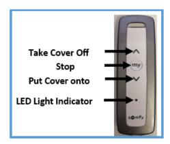
Note: User will identify on site that up and down arrows will change depending on orientation (left or right hand motor)
