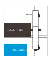
**TIP**: Ideally the roller tube should be positioned as close to the edge of the coping as possible. This positioning helps the cover lift up and directly onto the roller. Setting the roller too far back creates unnecessary drag and can cause the frames to tip forward.
